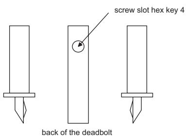
To reverse the latch bolt of the principal lock, firmly insert a flat-head screwdriver at an angle into the slot at the back of the latch bolt. When you push the screwdriver backwards the latch bolt is released and it can be reversed.
